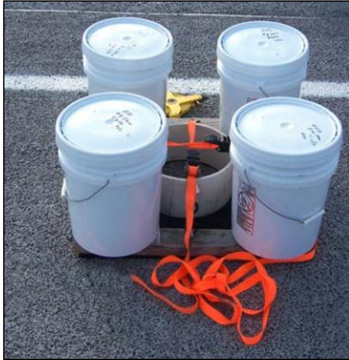
Figure 22 - Surface Infiltration Test Apparatus (Borst et al. 2010)
